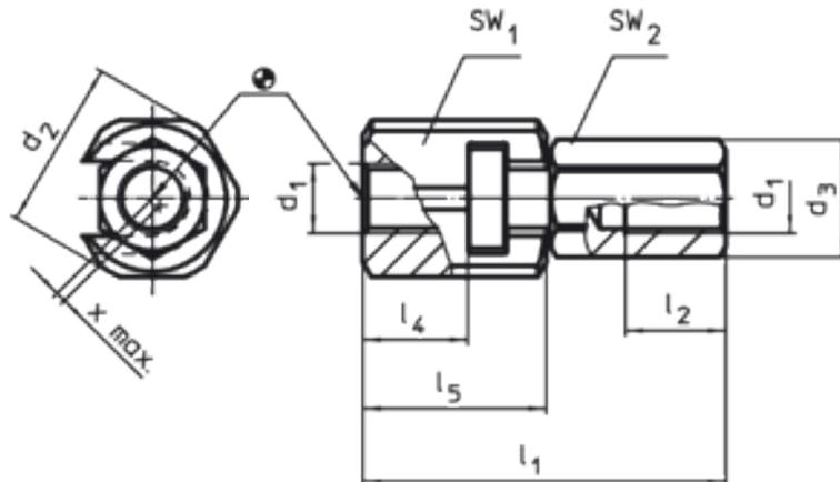
**AVEC ÉCROU D'ACCOUPLLEMENT**
